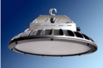
CircLED is a ø46cm round high bay fixture for general high bay applications such as auditoriums, exhibit halls, factories, distribution centres, and warehouses. SLP also have an IP66-rated version for harsh, wet environments. The housing, injection moulded with Covestro's thermally-conductive Makrolon® TC8030 polycarbonate, acts as a heat sink for the luminaire.
