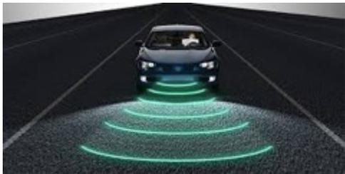
The company are working on lidar sensors with point cloud densities of 5 million to 20 million points per second in resolutions of approximately 720 vertical lines. The products are expected to be available in volume production early in 2019.
